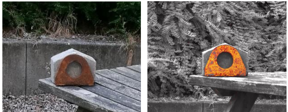
Left: Sample under investigation, Right: Sensor Output. Corroded areas are colored.
