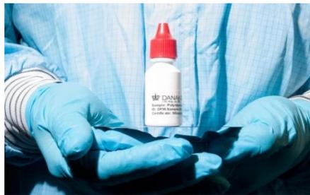
Photo: Bottle with a suspension of polystyrene particles for reference purposes. The average particle size is determined as part of the accredited services K09.101 og K02.102.
