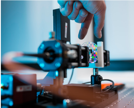
Portable scatterometer to characterize nanostructures at the fabrication sites.
