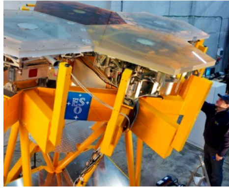
Assembled E-ELT mirror segments undergoing testing. Credit: ESO/H.-H. Heyer
